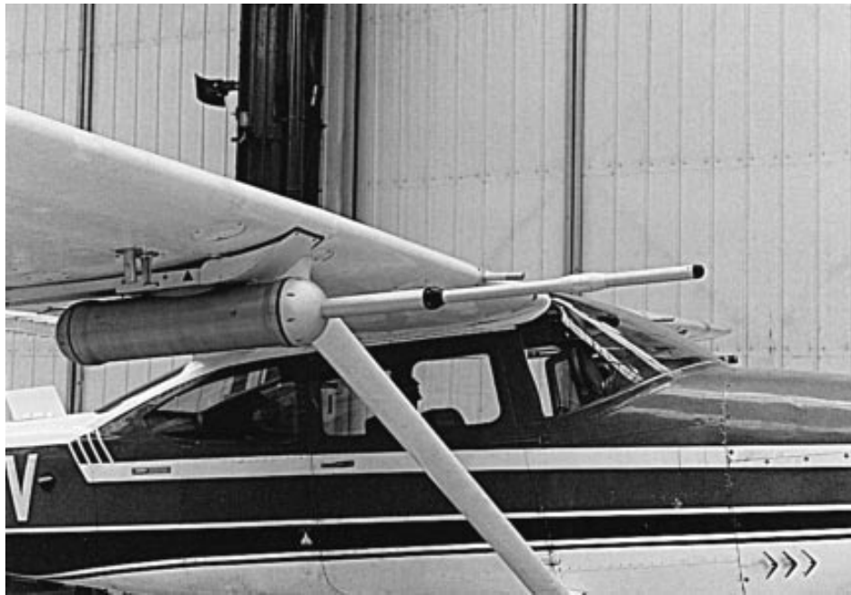
FIG. 1. The Cessna 182 aircraft showing the position of the five-hole probe.
