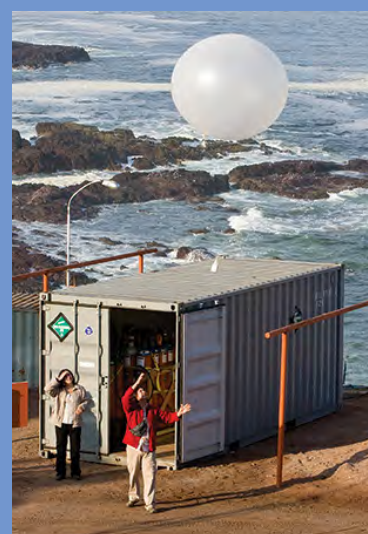
"Students from the Universidad de Arturo Prat, launch one of the four-times daily radiosondes from their shoreside campus in Iquique, Chile. Photo courtesy Carlye Calvin, UCAR"
