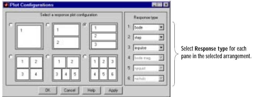
Figure 3-9: Using the Plot Configurations Dialog Box to Reconfigure the LTI Viewer
