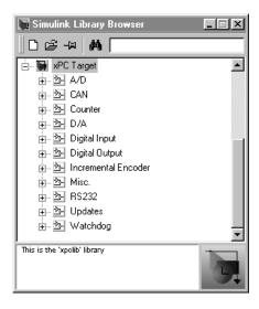
4 Open a function group. For example, to open the A/D group for ComputerBoards, double-click A/D, and then double-click ComputerBoards.
