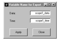
2 In the **Data** and **Time** text boxes, enter the name of the MATLAB variables to contain the data from the scope data package. Click the **Apply** button, and then click the **Close** button.
