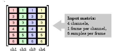
The **Number of channels** parameter specifies the number of independent channels (columns), N, in the matrix, and the block filters each channel independently over time. Frame-based operation provides substantial increases in throughput rates, at the expense of greater model latency.
