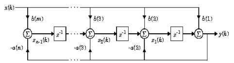
This is a canonical form that has the minimum number of delay elements. The filter order is max(m, n)-1.
