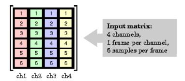
The **Number of channels** parameter specifies the number of independent channels (columns), N, in the matrix, and the block decimates each channel independently over time. Frame-based operation provides substantial increases in throughput rates, at the expense of greater model latency.
