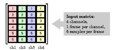
The **Number of channels** parameter specifies the number of independent channels (columns, N) in the matrix, and the block interpolates each channel independently over time. Frame-based operation provides substantial increases in throughput rates, at the expense of greater model latency.
