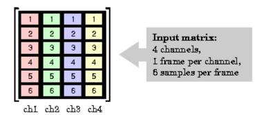
The **Number of channels** parameter specifies the number of independent channels (columns, N) in the matrix, and the block interpolates each channel independently over time. Frame-based operation provides substantial increases in throughput rates, at the expense of greater model latency.
