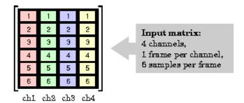
The Number of channels parameter specifies the number of independent channels (columns), N, in the matrix. The output is complex and has the same dimension and sample rate as the input (i.e., the FFT is computed at M frequency points for each channel).
