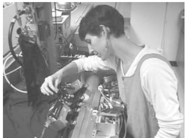
Sarah Masonis makes adjustments to the nephelometer, a new invention that measures scatter by atmospheric particles
